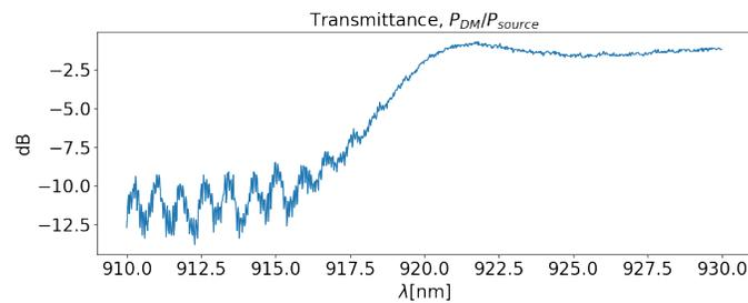
Figure 5. Dichroic mirror measured transmission spectrum.
