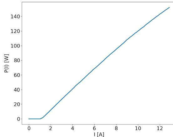
Figure 7. Coupled power against the driving current for the assembled module.
