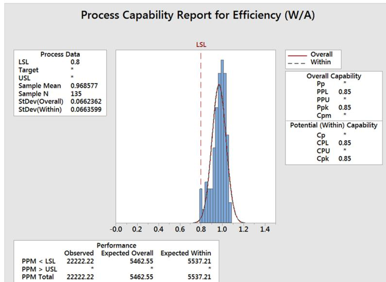
Figure 8: capability analysis for overall process efficiency, showing 98% observed yield
