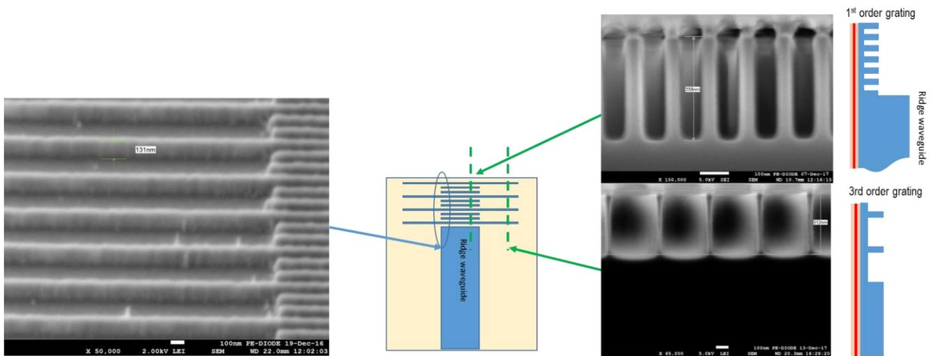
Figure 2: (center) schematic drawing of Bragg grating; (left) SEM top view of multiple order grating (right) SEM cross sections of first order and third order gratings
