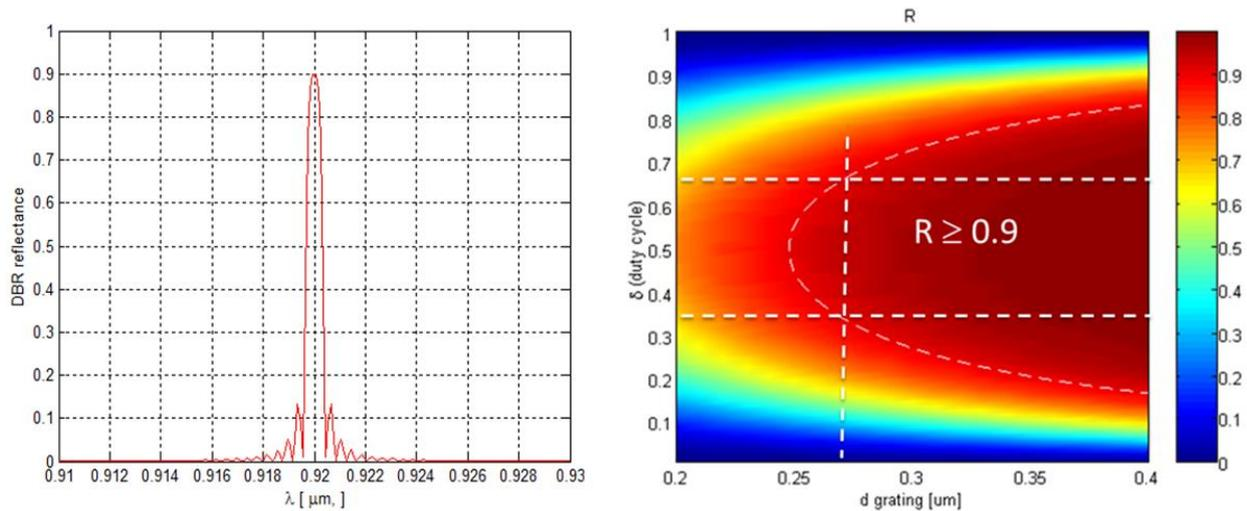
Figure 3: Calculation of the spectral reflectivity of the DBR section (*left*) and maximum of the reflectivity versus grating shape parameters: duty cycle  $\delta$ , and pitch  $d$  (*right*)
