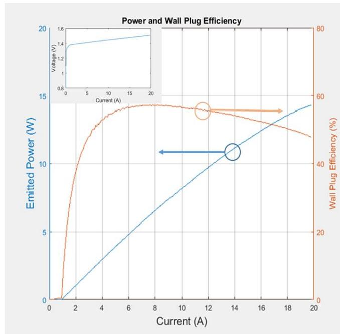
Figure 5: Emitted power and conversion efficiency (and diode voltage, inset) versus injected current (25 °C)
