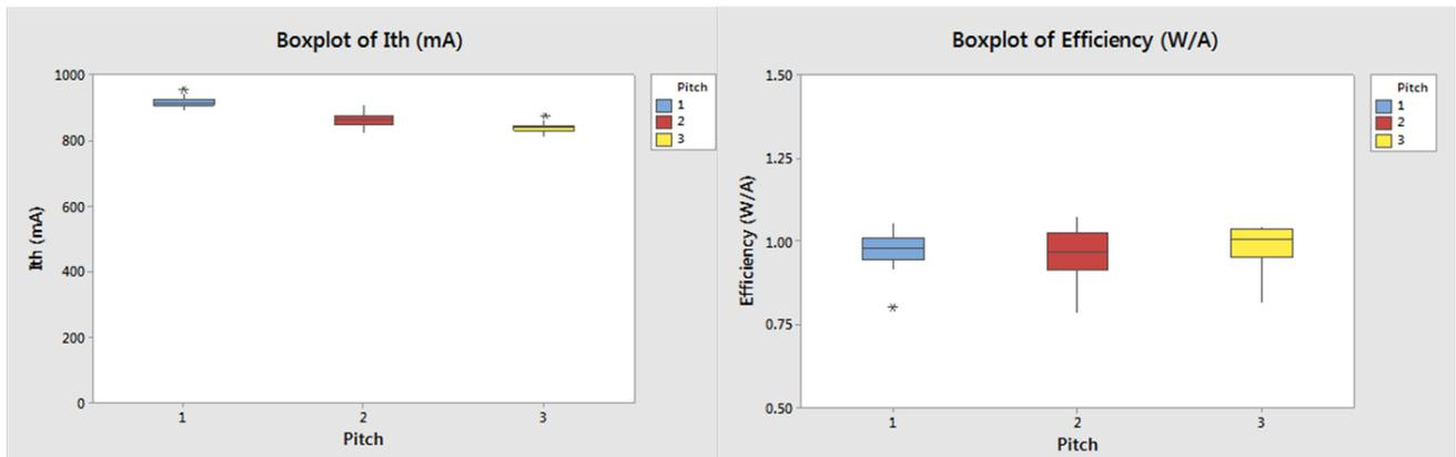
Figure 7: (left) box plot statistics of threshold current and (right) conversion efficiency (W/A)
