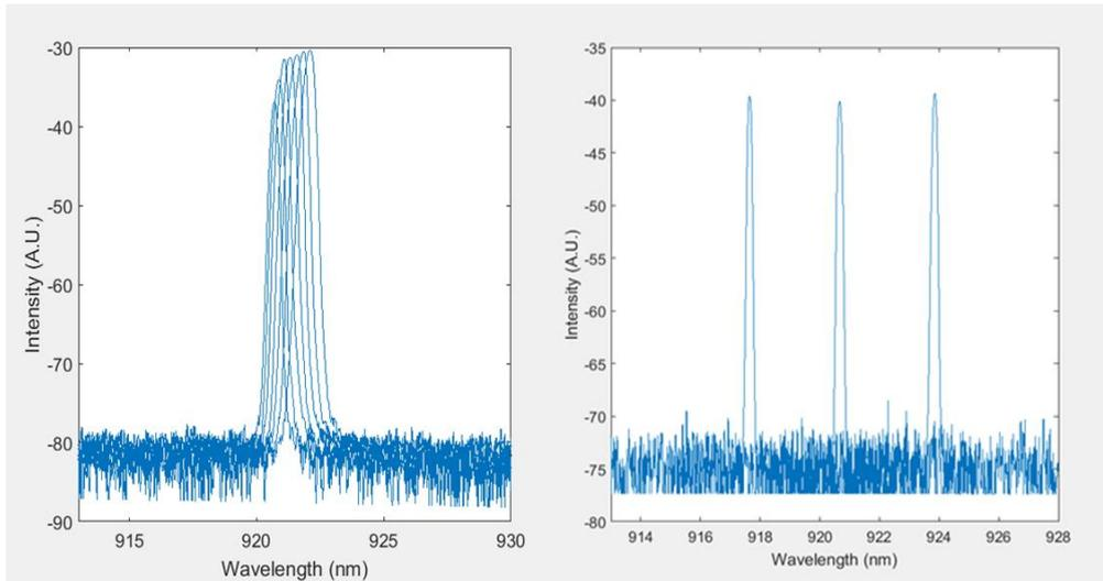
Figure 6: (left) emitted spectrum at 25 °C, 2-15A bias; (right) three wavelengths, 2.5 nm spaced emitted from the same wafer
