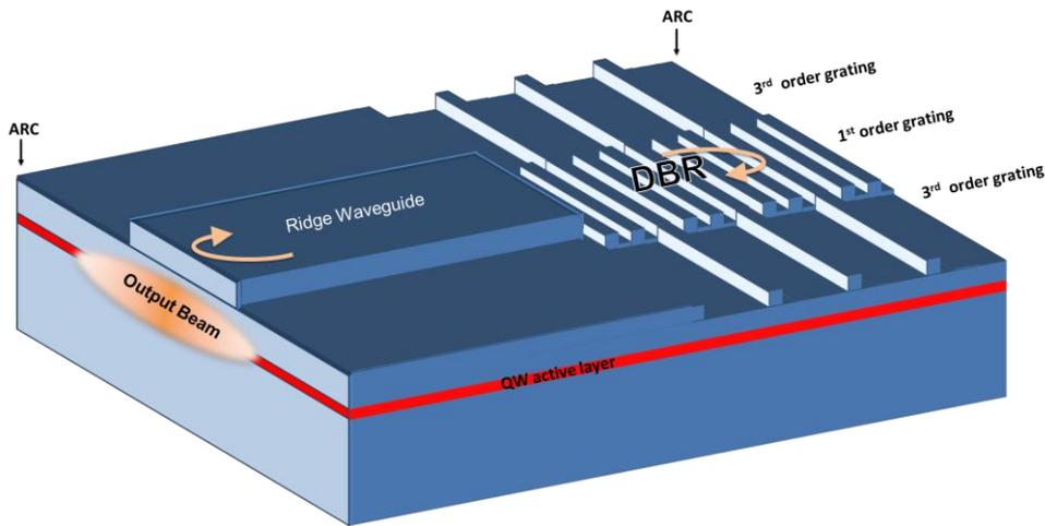
Figure 1: Schematic of the DBR high power laser diode
