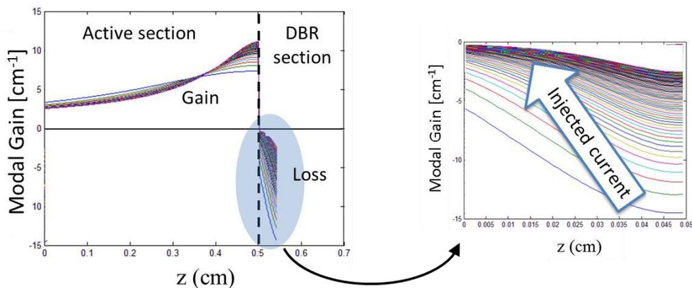
Figure 4: Calculation of the induced transparency in the DBR section
