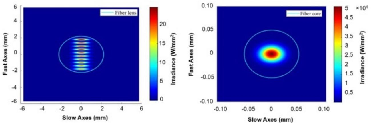
Figure 1: example of simulation with the optical layout of a stack of 10 emitters in 105 $\mu$ m fiber core: (*left*) beams stacking at focusing lens entrance; (*right*) focalized beam into the fiber core.
