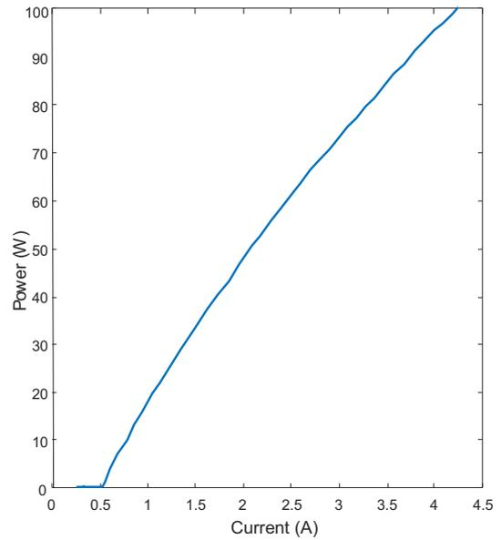
Figure 3: (left) the 100W module, under the power test; (right) the power / current characteristics, showing the output power in excess of 100 W
