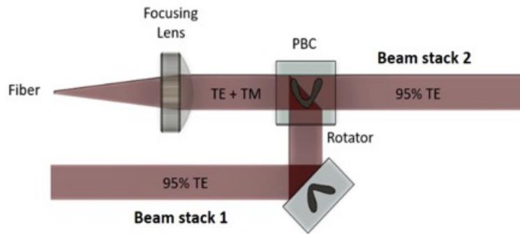
Figure 2: scheme of a polarization multiplexing. Two s-polarized beams pass through a Polarization Beam Combiner (PBC): one beam rotates its polarization plane by a half-wavelength plate, then its contribution is added to the other beam.
