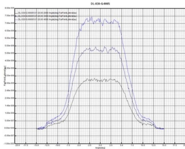
Figure 4: Far Field emitted by the module at 2, 3 and 4 A of bias current; a 0.15 N.A. at max power (filled by 95 % of emitted power) has been evaluated from the far field measurement
