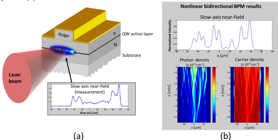
Figure 1: (a) slow-axis near field of a high-power broad-area semiconductor laser, (b) modelling results
