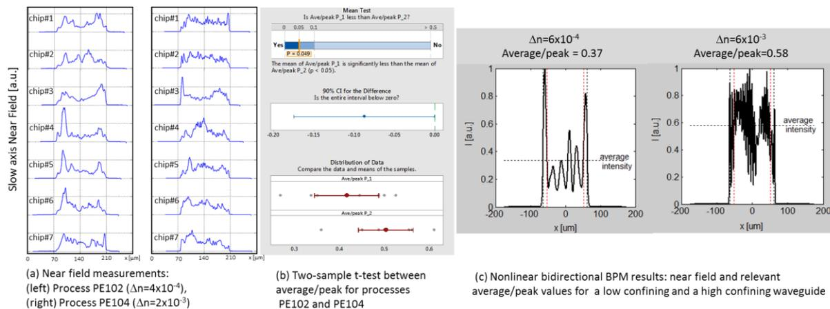
Figure 2: Slow-axis near-field measurements of laser chips belonging to wafer processes with different optical confinement (a), statistical comparison of average/peak values (b) and numerical calculations (c)
