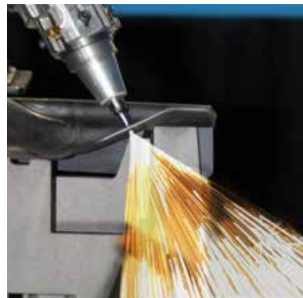
3D cutting high strength steel B-pillar using Convergent Photonics CF3000 Fiber laser.
