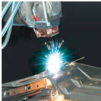
Laser welding titanium alloy using Convergent Photonics CM5000 CO 2 laser.
