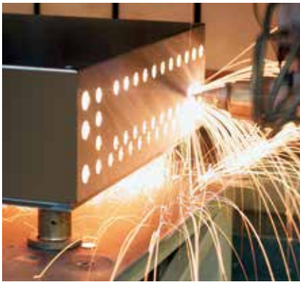
Laser cutting of stainless steel combustor using Convergent Photonics CX3000 CO 2 laser
