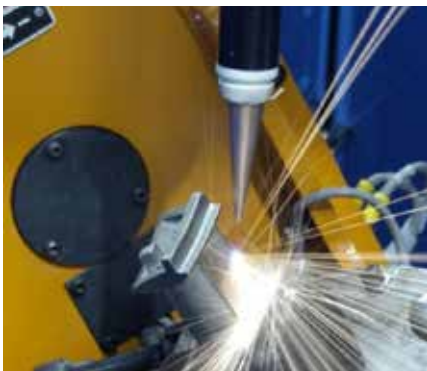
Laser drilling of aerospace turbine blade and vanes using Convergent Photonics CL50k Nd:YAG laser .
