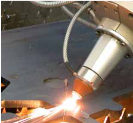
3D bevel cutting of 12mm mild carbon steel using Convergent Photonics CV5000 CO 2 laser .
