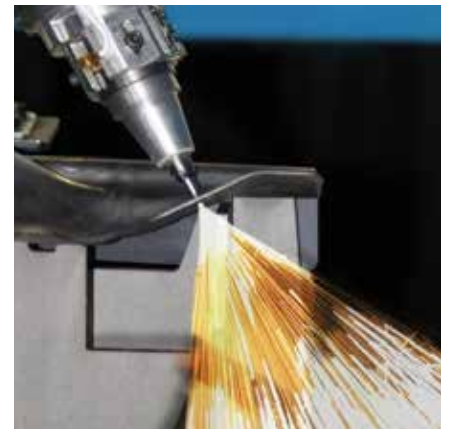
3D cutting high strength steel B-pillar using Convergent Photonics CF3000 Fiber laser.
