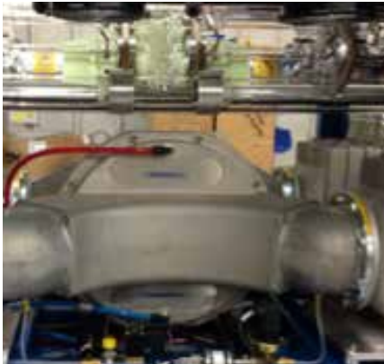
CP4000 CO 2 Laser retrofitted with new magnetic bearing turbine to improve performance and lower the cost of maintenance.
