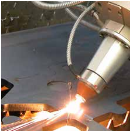
3D bevel cutting of 12mm mild carbon steel using Convergent Photonics CV5000 CO 2 laser .
