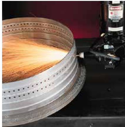
Precision cutting of an aircraft engine component using Convergent Photonics CL50k Nd:YAG laser.
