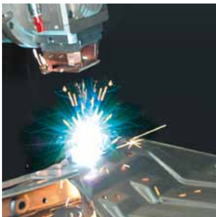
Laser welding titanium alloy using Convergent Photonics CV5000 CO 2 laser .
