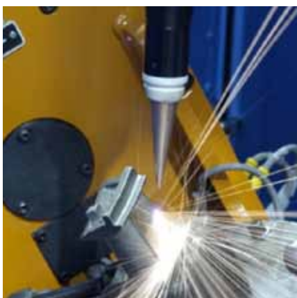
Laser drilling of aerospace turbine blade and vanes using Convergent Photonics CL50k Nd:YAG laser .
