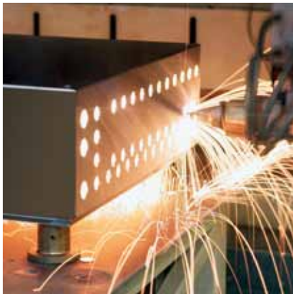
Laser cutting of stainless steel combustor using Convergent Photonics CX3000 CO 2 laser
